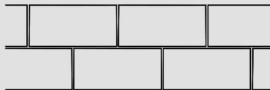
Typical Running Bond Concrete Masonry Units
