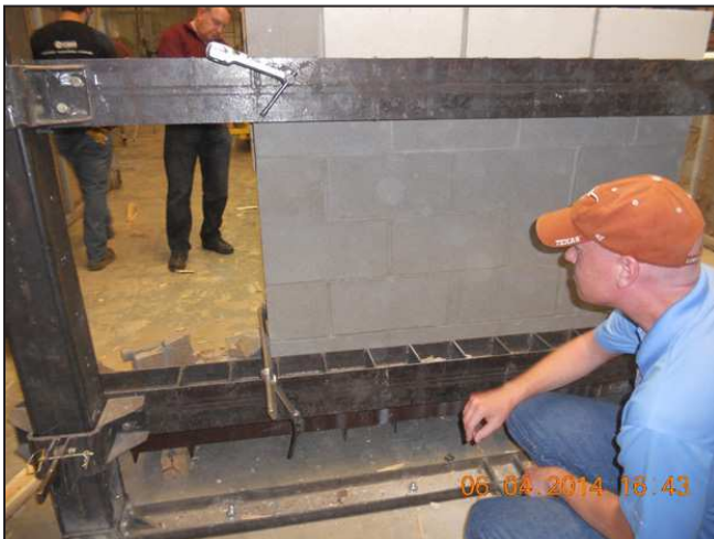
Figure 10 - Ben Harris inspecting the interior side of the CMU after the debris impact testing.
